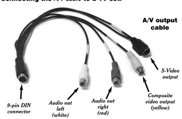
1. Plug the 9-pin DIN connector on the A/V output cable into the A/V output connector on the WinTV-PVR-350. This connector is "keyed" so you cannot plug it in backwards.
